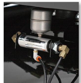
Tank drain automatically drains liquid from the air receiver
